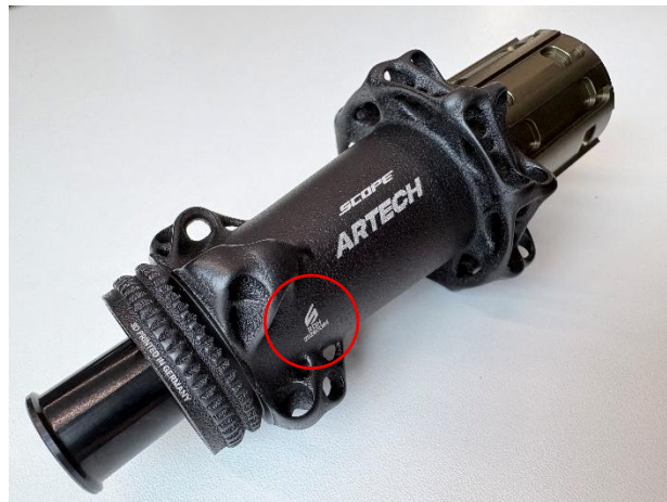
Figure 2: Serial number on Artech hub
