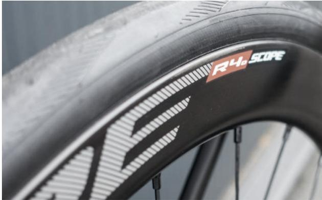
they are able to control all aspects of the parts used to build them. They are also able to develop their wheelsets with initially defined design requirements and characteristics in mind. For example, they have made the R4d wheelset as stiff as possible by making the distance between both flanges as wide as possible, resulting in an increased stiffness of the wheel. For the internals of the hub they use SKF bearings as a standard, whereas they also provide a CeramicSpeed upgrade for €500, -.
